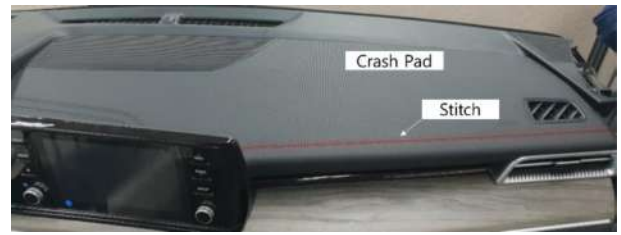
Fig. 2 A crash pad and stitches on it
