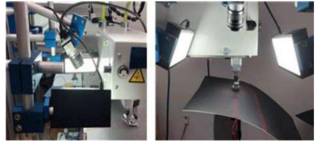
Fig. 3 The camera and dual LED lights for inspecting stitches
