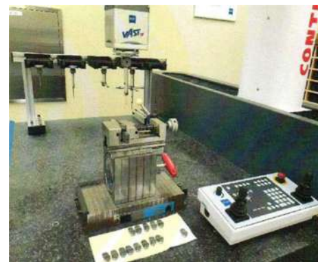
Fig. 19 Outside diameter measurement of Steering Stop product
