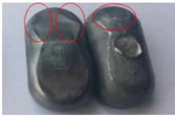
Fig. 16 Underfill defect of Steering Stop product at preform length 17 mm
