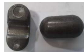
Fig. 18 Final trimming product of Steering Stop
