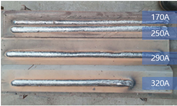
Fig. 13 Welding results of the proposed rotating welding torch for each welding currents
