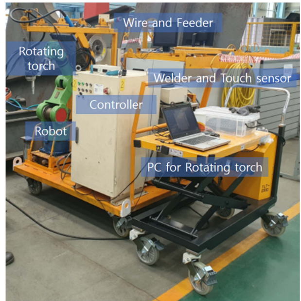
Fig. 12 The welding test bed for proposed rotating welding torch
