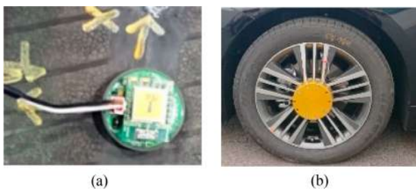
Fig. 3 Equipment module installed in tire: (a) Equipment module, (b) Battery
