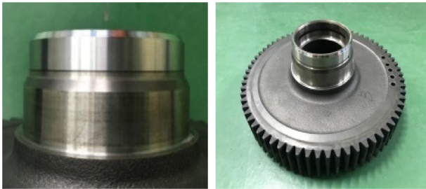
(b) Repaired gear
