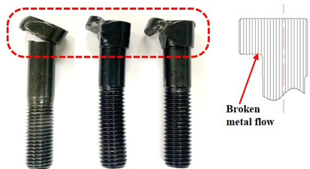
Fig. 3 Broken high-strength bolt head
