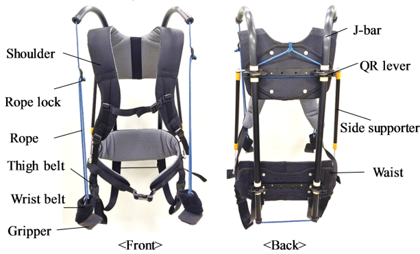
Fig. 1 Elements of the H-Frame
