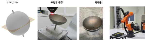
Fig. 14 3D Printing of pressure vessel
