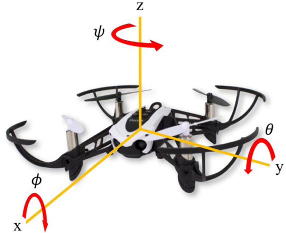
Fig. 1 The coordinate for mathematical model of the drone
