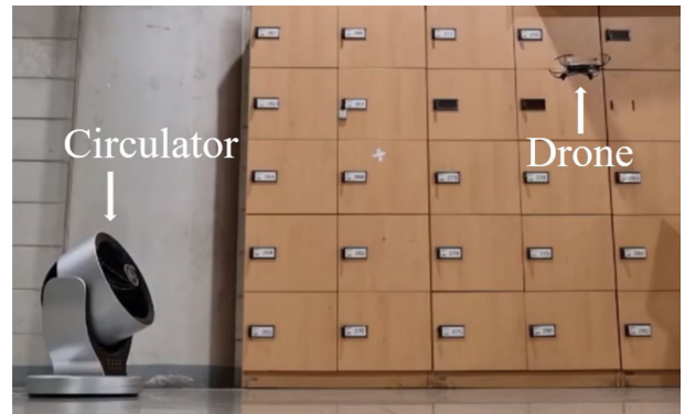
Fig. 8 Disturbance rejection experiments with a circulator
