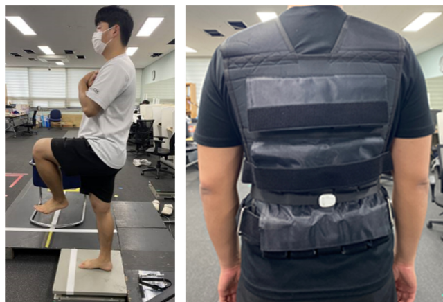
Fig. 2 One-leg standing test (left) and IMU sensor position (right)
