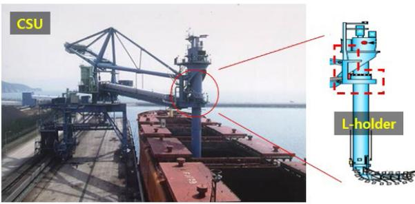
Fig. 1 Continuous ship unloader
