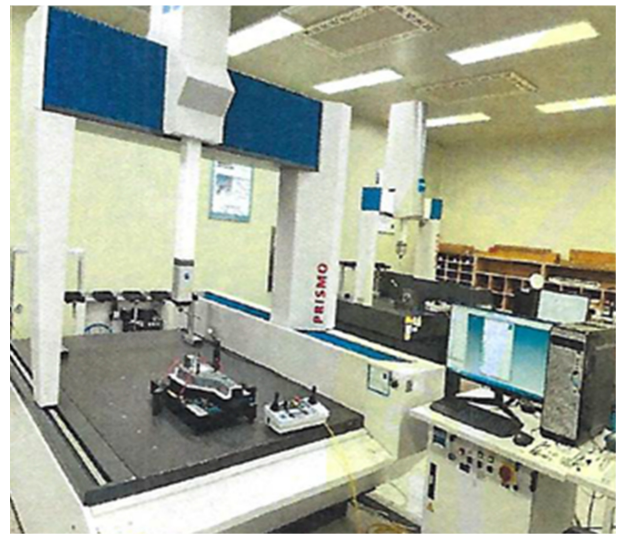
Fig. 14 Measurement scene of 3D coordinate measuring machine for radiator support parts
