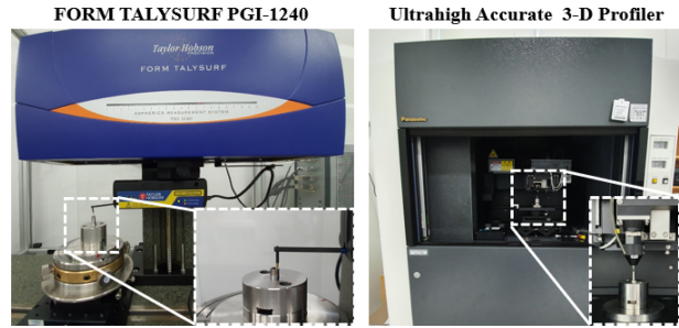
Fig. 3 Surface profile measurement systems (Left is PGI-1240 of Taylor Hobson, right is UA3P of PANASONIC)
