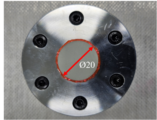
Fig. 1 Germanium (Ge) sample with machining jig
