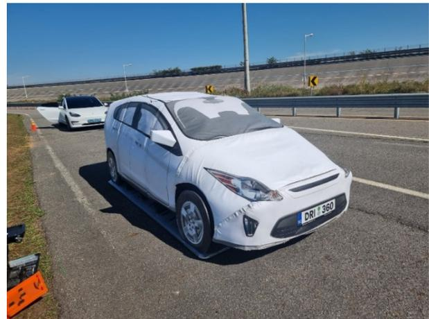
Fig. 2 Guided vehicle target robot with dummy
