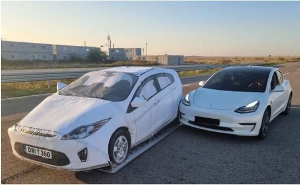
Fig. 4 Guided vehicle target robot test
