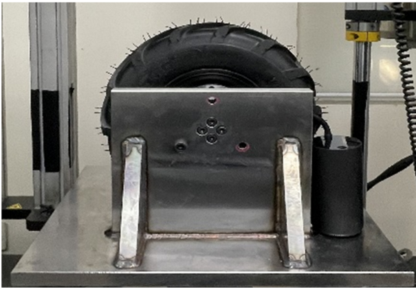
Fig. 3 Experimental setup for tire characteristics
