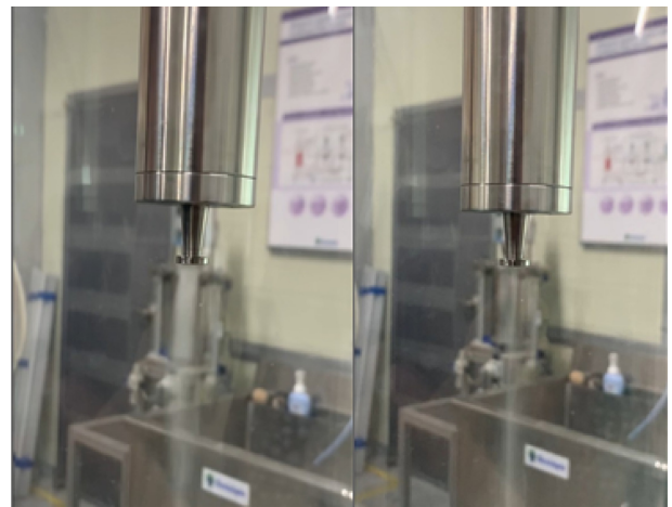
Fig. 2 Mist spraying at ultrasonic nozzle (SonoMist™)
