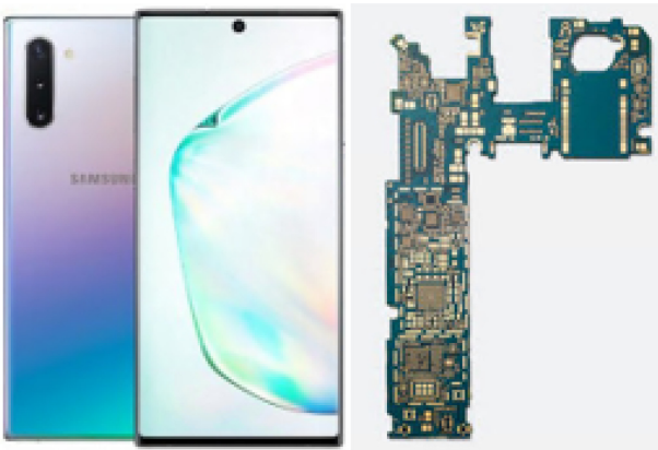
Fig. 1 Premium smart phone and main PCB board
