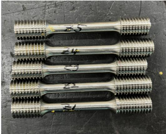
(a) Before tensile test specimens (Z-direction)
