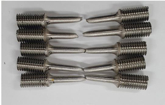
(b) After tensile test specimens (Z-direction)
