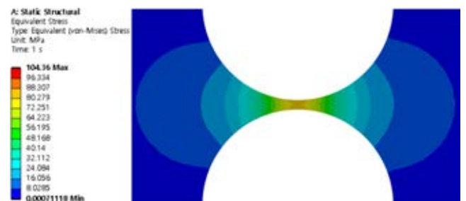
Fig. 5 Stress distribution of a 1-D circular flexure hinge when axially extended
