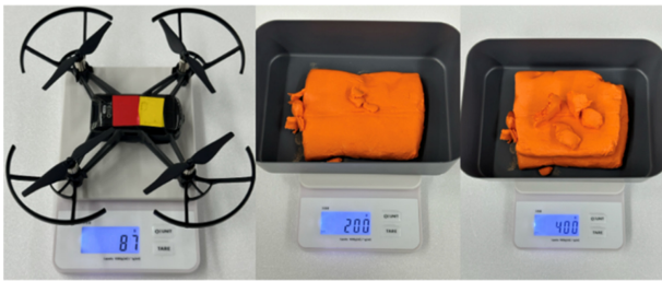
Fig. 7 Experimental environment for payload measurement of drone pose alignment manipulator
