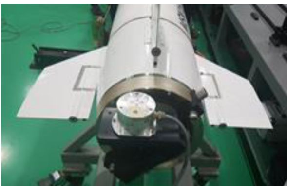
Fig. 14 Measurement for an absolute position of missile base
