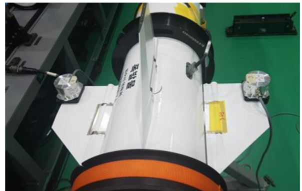
Fig. 12 Measurement for an assembling error of control fins
