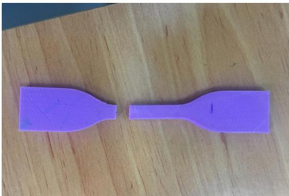
Fig. 3 Specimens after tensile test
