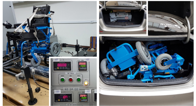
Fig. 12 Fatigue strength test in accordance with ISO 7176-8 (left) and foldable electric wheelchair loaded in the car trunk (right)
