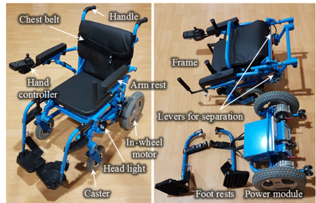
Fig. 10 The prototype of foldable wheelchair with separable power module (left), folded electric wheelchair and separable power module including battery, in-wheel motor and controller (right)
