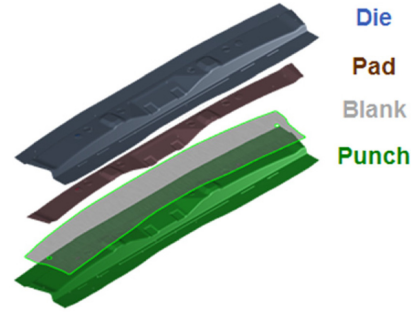
Fig. 2 Finite element model of the stamping analysis
