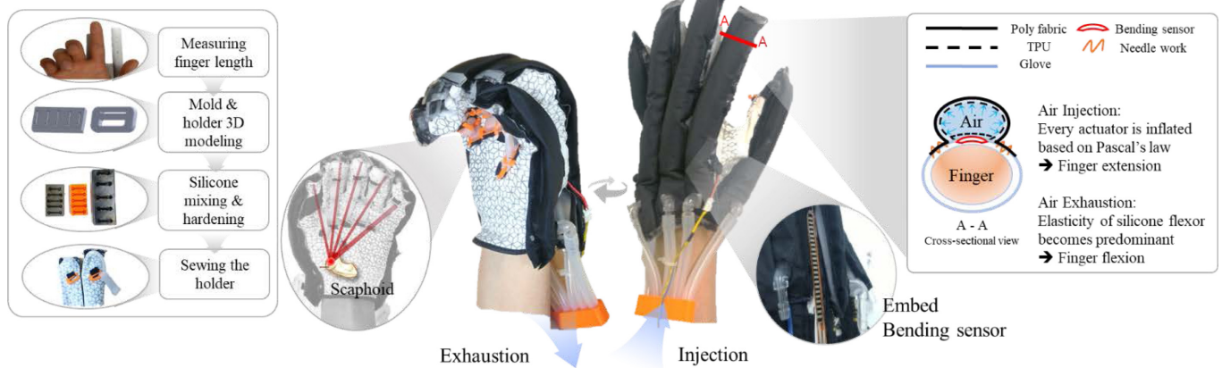
Fig. 1 Components of the air pocket glove, operation principle and overall manufacturing process
