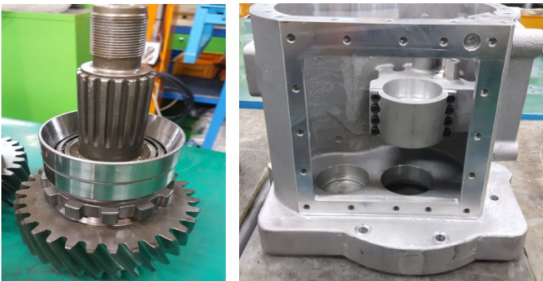
Fig. 11 Manufactured output gear and housing
