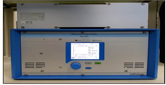
Fig. 9 DAQ and multichannel charge amplifier
