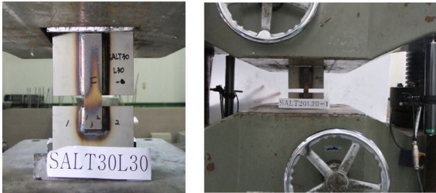
(b) Set-up of test specimens and transducers (LVDTs)
