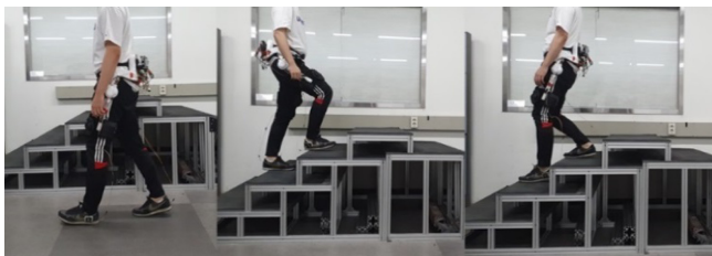
Fig. 7 Locomotion modes and walking test platform (Left: LW, mid: SA, right: SD)
