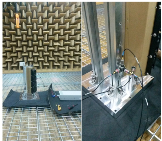
Fig. 12 Equipment composition for structure borne noise test of side fan assembly
