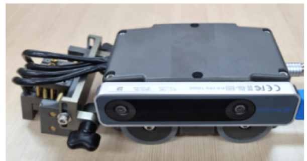
Fig. 7 Attaching the IMU sensor to the scanner
