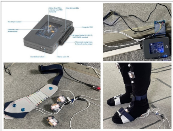
Fig. 3 Data acquisition system by NI myRIO box
