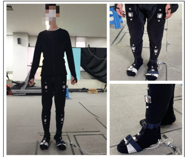
Fig. 4 Attachment of gait acquisition sensor system and marker
