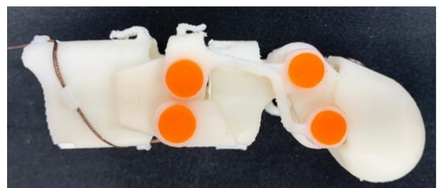
Fig. 12 The prosthetic finger using a 3D printer
