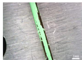
(d) Photograph of wear and defect of PTFE applied mold after 100 cycles
