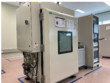
Fig. 12 Test equipment for rapid temperature change
