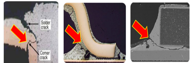
Fig. 2 Main failure mode of electronic control unit
