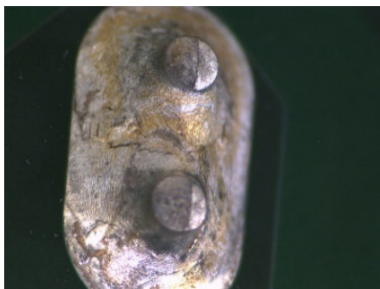
Fig. 13 Circular cracks caused by thermal shock cycle test with rapid temperature change
