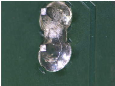
Fig. 11 Circular crack generated by normal mode thermal shock cycle test
