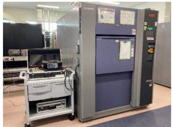
Fig. 6 Test equipment of thermal shock cycle
