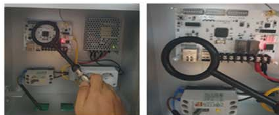
(e) Measurement result of wireless gateway controller using noise scanner
