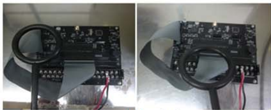
(a) Measurement result of wireless heat pump electric heater controller using noise scanner
