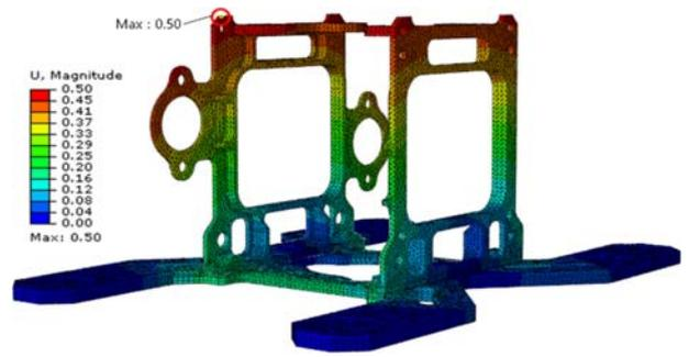
Fig. 14 Deformation of modified support structure
