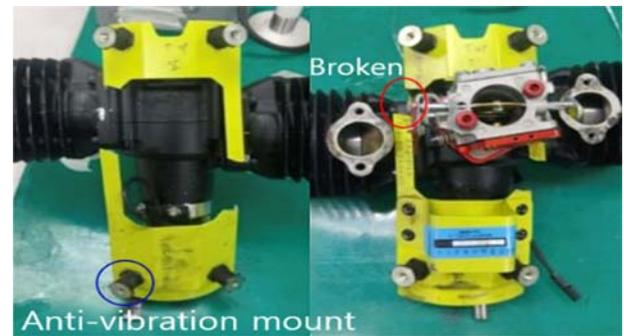
Fig. 2 Failure example of engine-generator support structure
