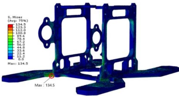
Fig. 13 Effective stress distribution of modified support structure
