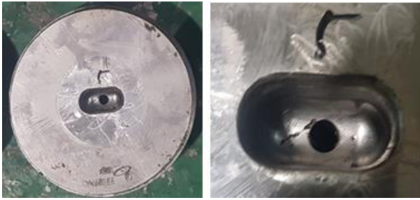
Fig. 6 Cold forging tool breakage of Steering Stop product before improvement
