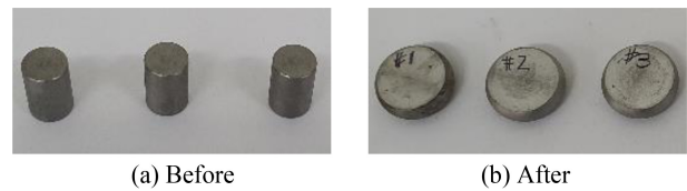
Fig. 3 Test specimens of before and after compression test
