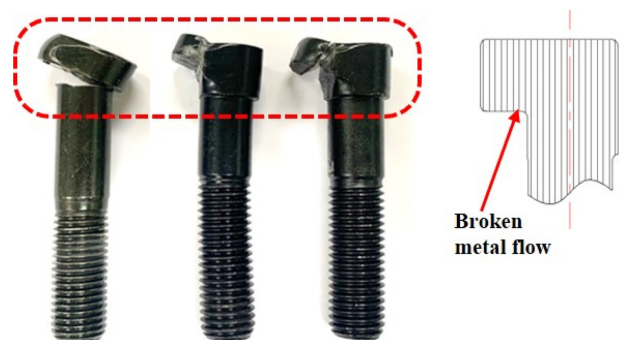
Fig. 3 Broken high-strength bolt head
