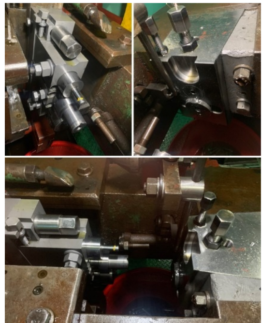
Fig. 11 Eccentric bolt forging process mold mounted on a heading machine
