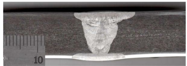
Fig. 1 Inconel 617 alloy welded block
