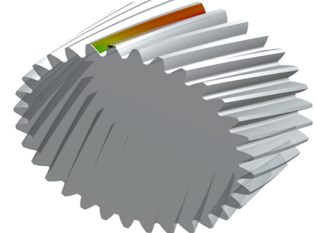
Fig. 10 Stress distribution on tooth modification after
