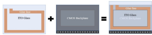
Fig. 2 Illustration of the process step involving the alignment and lamination of ITO glass onto a CMOS backplane chip
