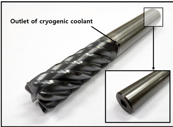
Fig. 2 Cryogenic machining tool including indirect spraying system
