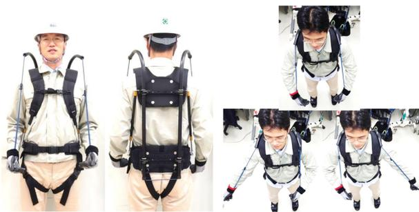
Fig. 2 How to wear the H-Frame
