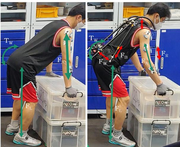
Fig. 3 Comparison of forces acting on the H-Frame
