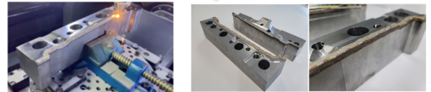
Fig. 13 3D Printing of cold press shear mold using developed CAM S/W
