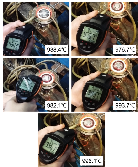
Fig. 2 Measurement temperature of park gear during induction heating
