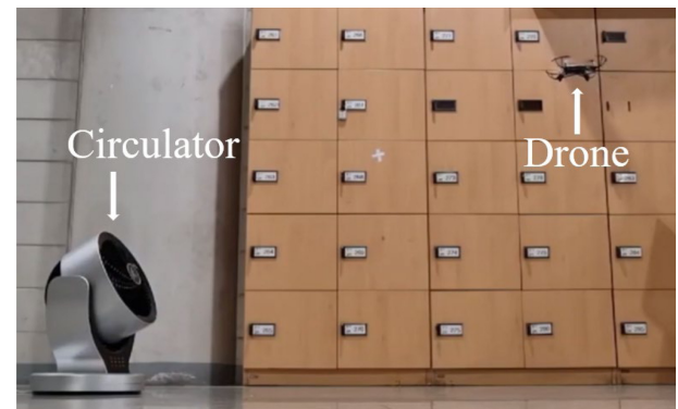
Fig. 8 Disturbance rejection experiments with a circulator
