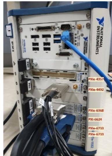
Fig. 5 NI real-time hardware (PXIe-8135)
