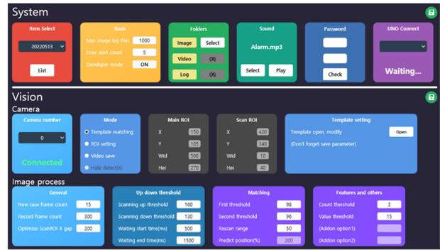
Fig. 2 Integrated graphic user interface for the proposed vision system
