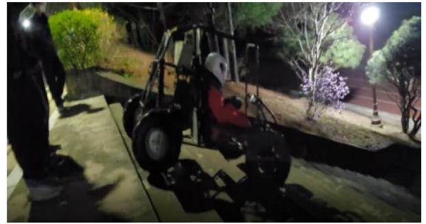
Fig. 6 Stair drop experiment
