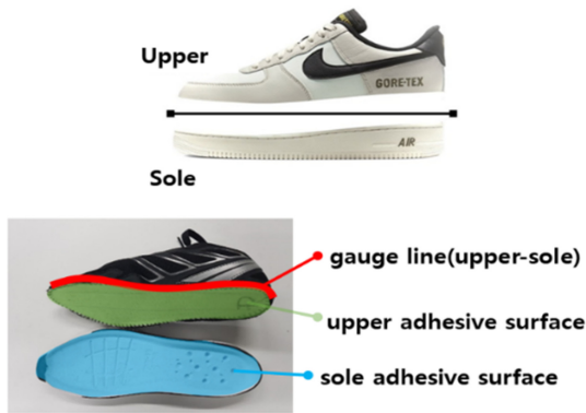
Fig. 1 Structure of shoes
