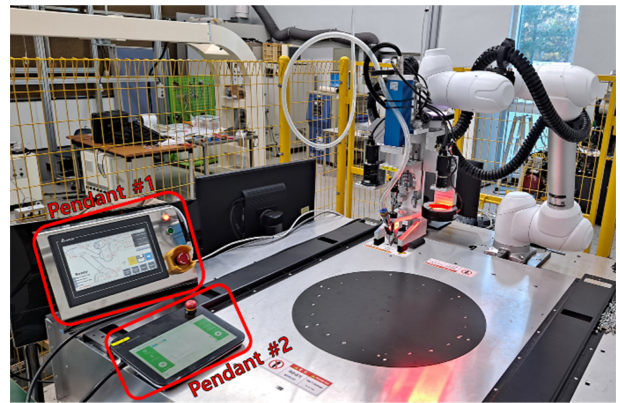
Fig. 4 Overview of screwing automation robot system
