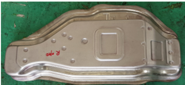
Fig. 12 Final blank shape of forming/drawing process
