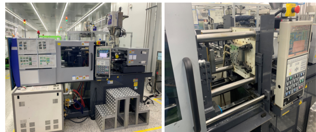
Fig. 4 Experimental set-up for plastic injection molding (SE50D, sumitomo)
