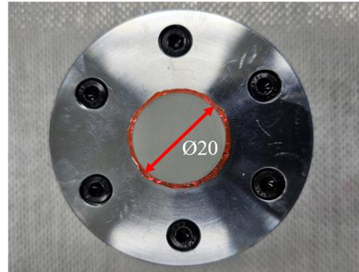
Fig. 1 Germanium (Ge) sample with machining jig
