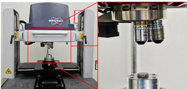
Fig. 4 White light scanning interferometer
